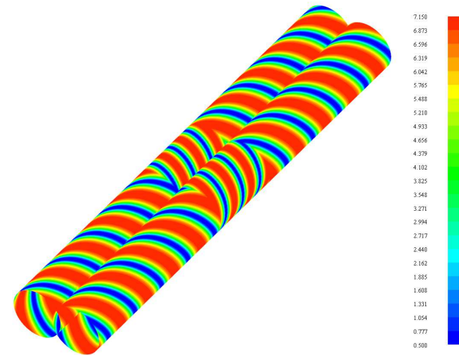
Thickness information mapped on 2.5D Hele-Shaw FEM meshes
