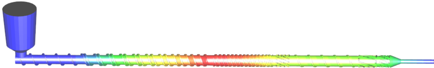
Fig.11 Predicted pressure distribution ( Min:0MPa,Max:30MPa)
